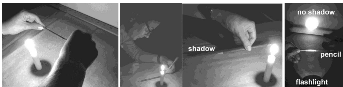
Fig. 3. Left: Moving a pencil near a candle while observing its shadow. Left middle: marking the shadow beneath a pencil. Right middle: The pencil’s shadow lengthens as it is raised. Right: a pencil casts no shadow inside a flashlight’s beam.
